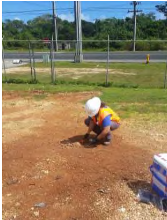
Soil Sample Collection at Oil Stained Location
