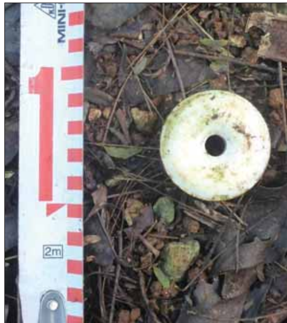
Figure 38. ISO-2 electrical insulator.
