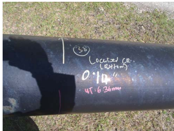
Localized corrosion at 6H00
